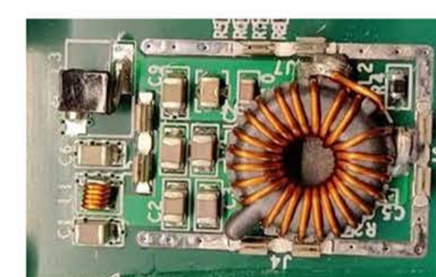
耐辐照电源转换单元 DC/DC converter (bPOL12v) with radiation tolerance
