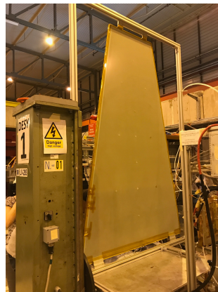
Figure 7.3: Top) Picture of the CMS GE1/1- \mu RWell prototype. Bottom) Picture of the CMS GE2/1 sector with two M4 \mu RWell prototypes.
